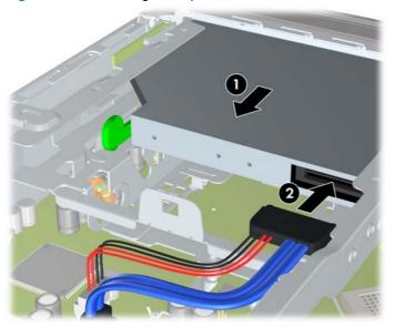
Figure 7-18 Installing the Optical Drive
